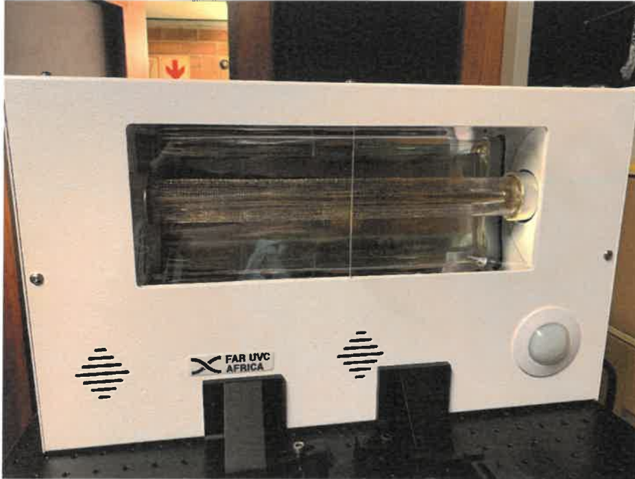
Figure 1: Photograph of the UVGI device. The device is a wall mount unit with a 150W Far-UVC lamp with crystal quartz filters and a motion sensor. The motion sensor was bypassed.
